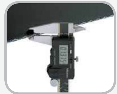
Measure belt thickness.
