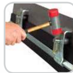
Quick adjustment by using the locking wedges on the clamp pins
